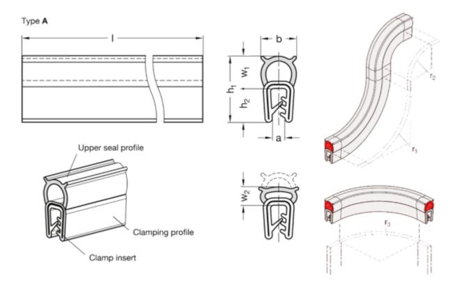
$$\begin{array}{lll} a & = 0.8 - 2.5 \\ b & = 8.5 \\ h1 & = 15.5 \\ h2 & = 9 \\ I \text{ (Meter)} = 20 \\ r1 & = 80 \\ r2 & = 50 \\ r3 & = 20 \\ \end{array}$$
